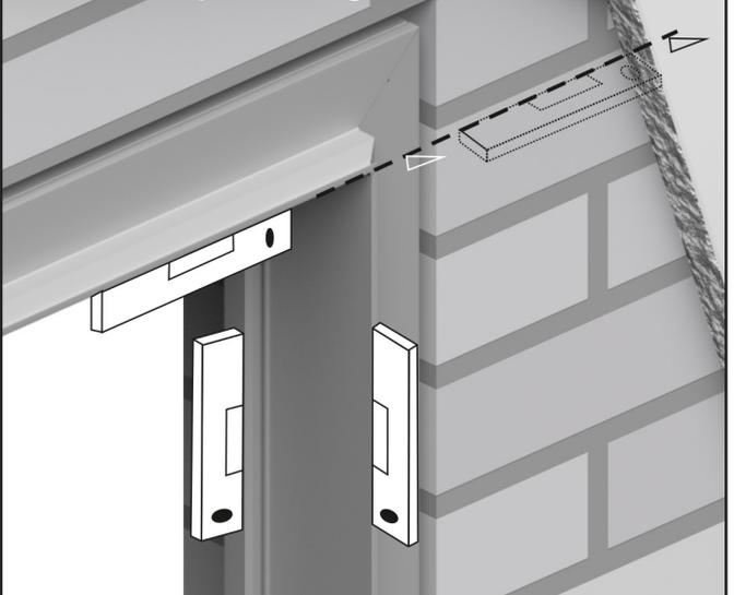
Wedge the aligned door frame in the opening
