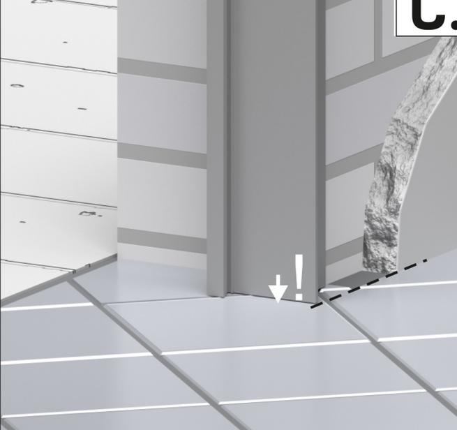
Measure vertical and horizontal alignment of the door frame. If necessary, adjust the alignment
